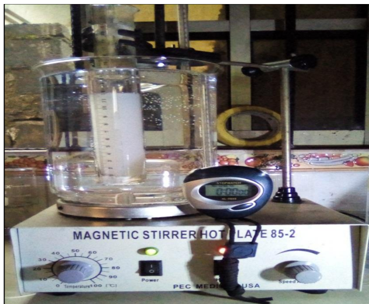
Plate 1: Precipitate Sedimentation Measurement Apparatus- The PreSed Meter.
